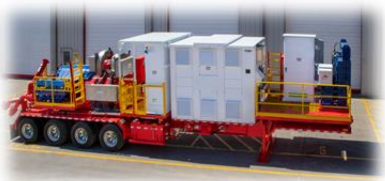
Stewart & Stevenson built electric frac unit
