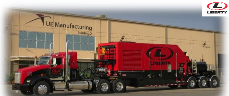
UE Manufacturing built quiet frac unit
